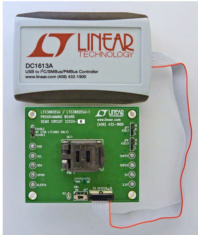
Figure 3. DC1613A Ribbon Cable Installation
