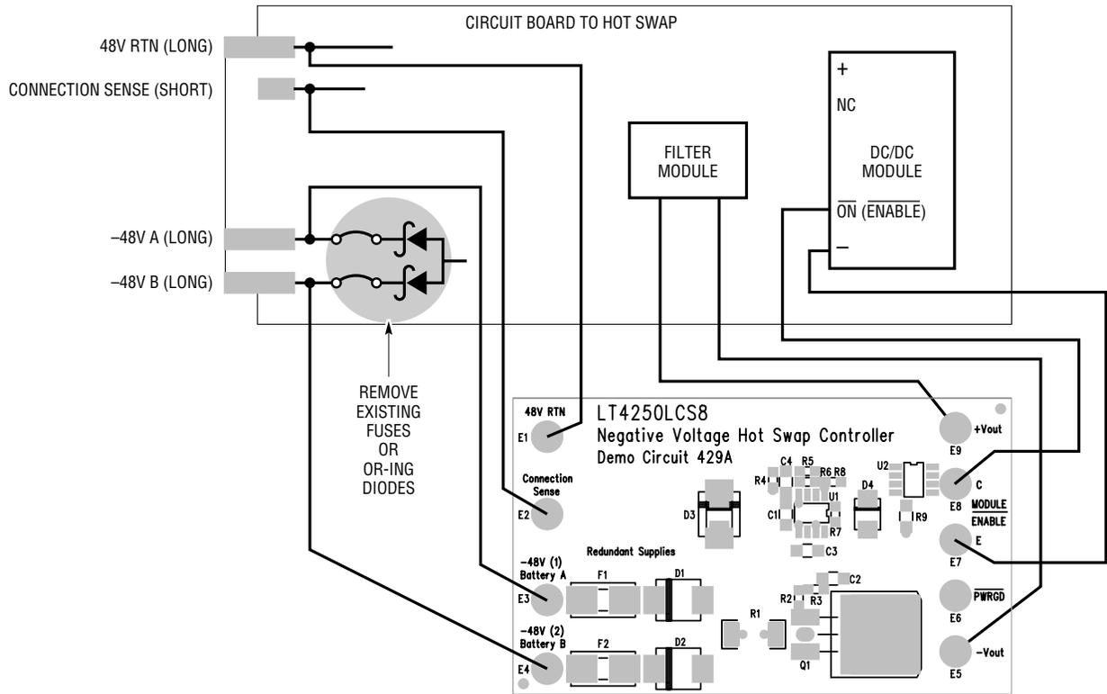
Figure 2. Setup for Circuit Board with Input Filter
