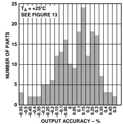
Figure 12. Output Accuracy Distribution,  $V_{OUT} = 2.8V$
