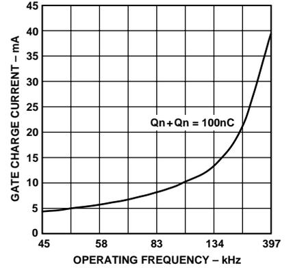
Figure 6. Gate Charge Supply Current vs. Operating Frequency
