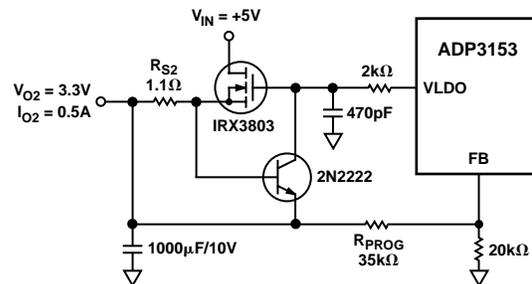
Figure 14. Linear Regulator with Overcurrent Protection
