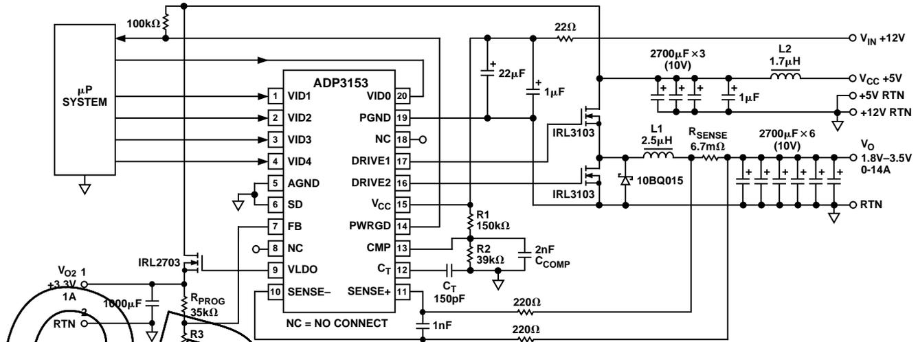
Figure 2. Typical VFM8.2 Compliant Core DC/DC Converter Circuit
