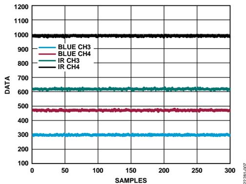
Figure 6. Background Signal Appearing on ADPD188BI Readings
