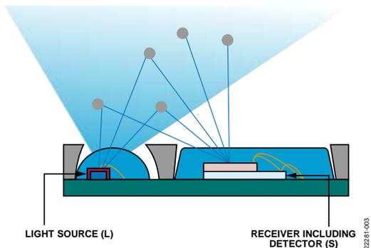
Figure 2. Backscattering of Light from ADPD188BI LEDs
