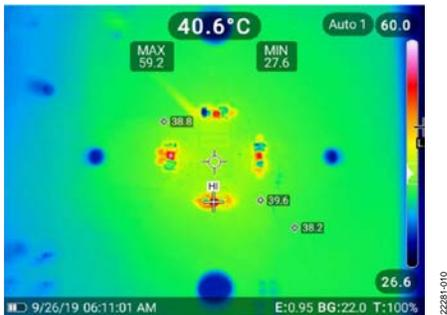
Figure 9. Infrared Image of the CN-0537 Heating Resistors
