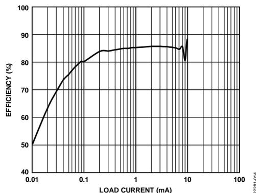
Figure 13. LT8410 Efficiency vs. Load Current Plot
