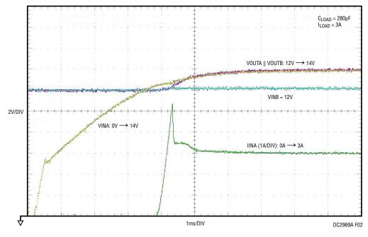
Figure 2. VINA and VINB Ideal Diode-OR: VINB is at 12V while VINA turns on from OV to 14V
