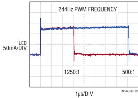
Figure 3. DC2630A PWM Dimming Using I<sup>2</sup>C Settings for 1250:1 and 500:1 Dimming Ratios
