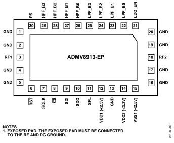
Figure 3. Pin Configuration
