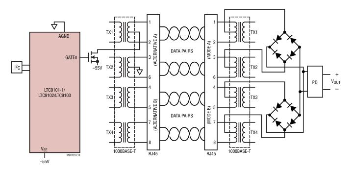
Figure 10. 2-Pair, Alternative A (Endpoint), Power over Ethernet Single-Signature PD System Diagram
