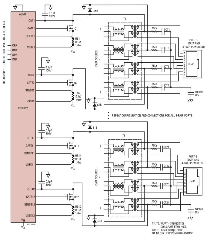
Figure 32. Alternative A (MDI-X) and B (S), 4-Pair, 1000BASE-T, IEEE 802.3bt, Type 3 or Type 4 PSE, Ports 1 and 6 Shown
