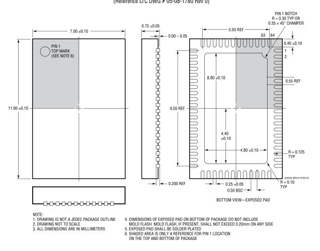
UKJ Package 64-Lead Plastic QFN (7mm × 11mm) (Reference LTC DWG # 05-08-1780 Rev 0)
