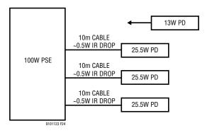
Figure 24. 100W PoE System with 10m Cables
