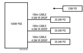
Figure 23. 100W PoE System with 100m Cables
