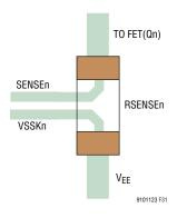
Figure 31.  $R_{\mbox{SENSE}}$  Kelvin Connections
