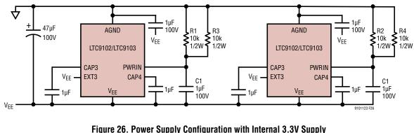
Figure 26. Power Supply Configuration with Internal 3.3V Supply
