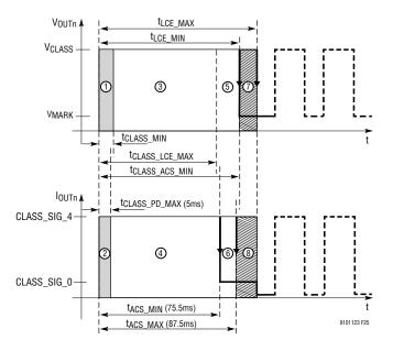
Figure 25. Autoclass Negotiation, Voltage and Current
