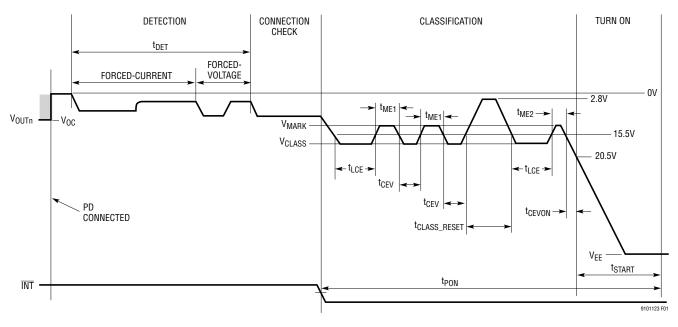
Figure 1. Detect, Class and Turn-On Timing, 4-Pair Port, Primary Alternative, Auto or Semi-Auto Mode
