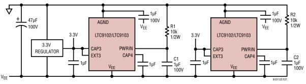
Figure 27. Power Supply Configuration with External 3.3V Regulators
