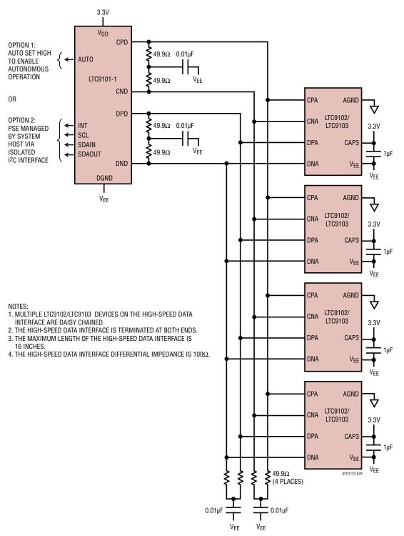
Figure 29. LTC9101-1/LTC9102/LTC9103 Proprietary Direct Connection Scheme
