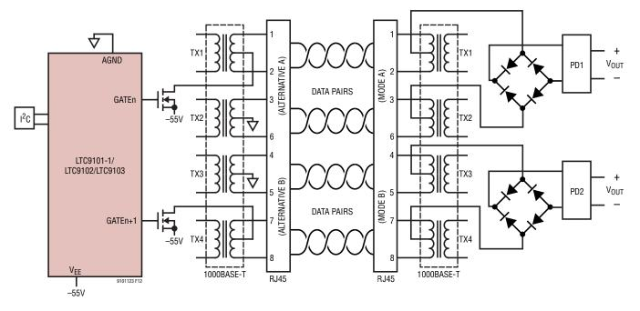
Figure 12. 4-Pair Power over Ethernet Dual-Signature PD System Diagram
