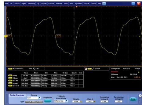
Figure 3. D<sub>OUT1-</sub> and D<sub>OUT1+</sub> with a 1.25 GHz Clock, Differential
