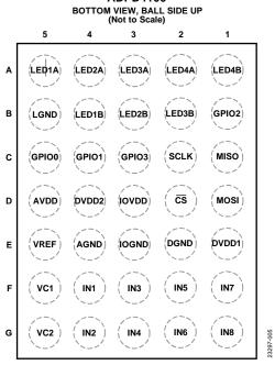
Figure 4. ADPD4100 Pin Configuration
