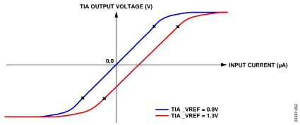
$Figure~51.~Illustration~of~Trigger~Points~for~TIA~Ceiling~Detection~for~TIA\_VREF = 0.9~V~and~TIA\_VREF = 1.3~V,\\ Points~Marked~by~Black~Crosses~TIA\_VREF = 0.9~V~and~TIA\_VREF =$
