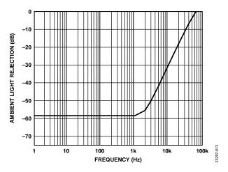
Figure 12. Ambient Light Rejection vs. Frequency
