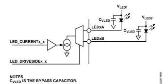
Figure 18. Block Diagram of LED Driver Output Pair
