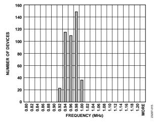
Figure 14. 1 MHz Clock Frequency Distribution, Untrimmed
