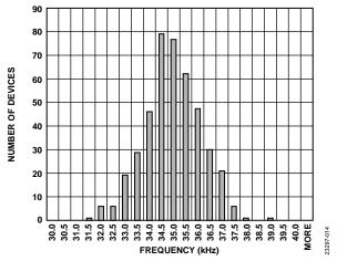
Figure 13. 32 kHz Clock Frequency Distribution, Untrimmed
