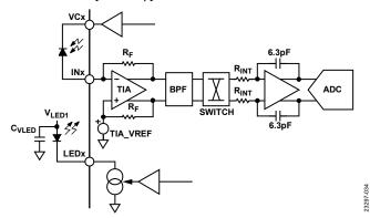
Figure 34. Typical PPG Measurement Circuit
