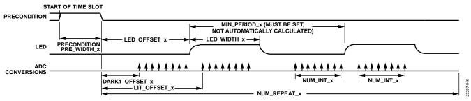
Figure 46. One-Region Digital Integration Mode Timing Diagram
