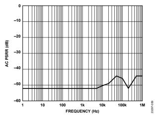
Figure 7. AC PSRR vs. Frequency
