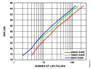
Figure 10. SNR vs. Number of LED Pulses in Continuous Connect Mode,  $C_{PD} = 70$  pF, Integrator Input Resistor = 400 k $\Omega$ , 90% Full Scale
