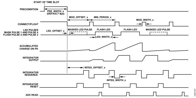
Figure 37. Four-Pulse Float Mode Operation
