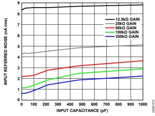
Figure 9. Input Referred Noise vs. Input Capacitance, Integrator Input Resistor = 400 k $\Omega$
