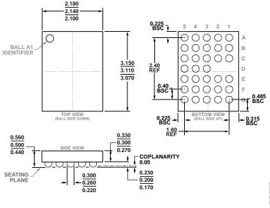
Figure 59. 33-Ball Wafer Level Chip Scale Package [WLCSP] (CB-33-1) Dimensions shown in millimeters
