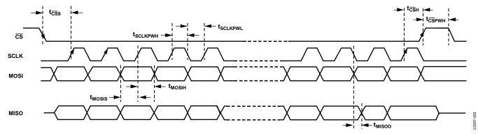
Figure 3. SPI Timing Diagram for the ADPD4100
