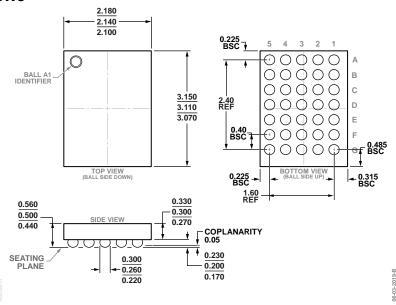
Figure 58. 35-Ball Wafer Level Chip Scale Package [WLCSP] (CB-35-2) Dimensions shown in millimeters
