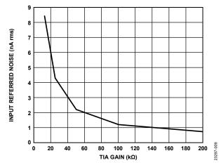
Figure 8. Input Referred Noise vs. TIA Gain,  $C_{PD}$  = 70 pF, Integrator Input Resistor = 400 k $\Omega$
