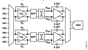
Figure 16. Analog Signal Path Block Diagram
