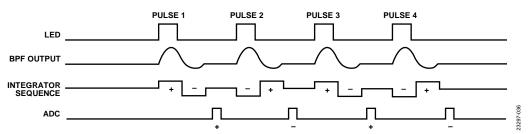
Figure 36. Diagram of Integrator Chopping Sequence
