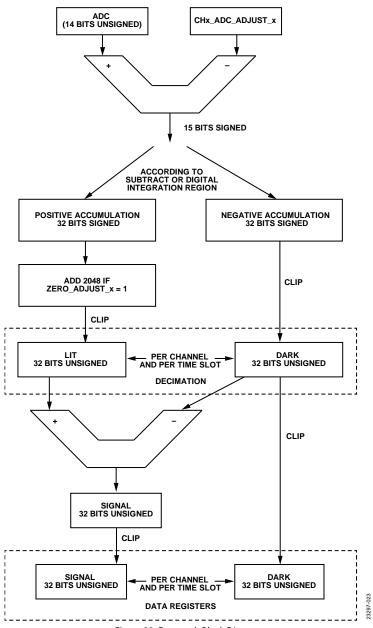
Figure 23. Datapath Block Diagram
