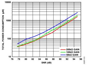
Figure 11. Total Power Consumption vs SNR in Continuous Connect Mode Including LED Power,  $C_{PD} = 70$  pF, Integrator Input Resistor = 400 k $\Omega$ , ODR = 25 Hz, CTR = 150 nA/mA, LED Supply Voltage = 4 V, 90% of Full Scale
