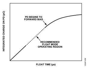
Figure 38. Integrated Charge on the Photodiode (PD) vs. Float Time
