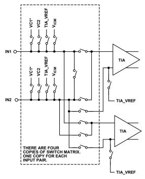
\*ALL BIAS CONNECTIONS SHOWN ARE ONLY AVAILABLE DURING SLEEP AND PRECONDITIONING PERIODS. THE SWITCHES TO THESE BIAS LEVEL ARE OPEN DURING TIME SLOTS WITH THE RESPECTIVE INPUTS SELECTED.
