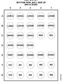
Figure 5. ADPD4101 Pin Configuration
