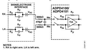
Figure 52. Circuit for Measuring Single-Lead ECG with the ADPD4100/ADPD4101
