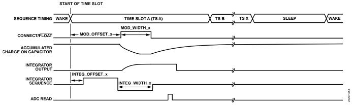
Figure 53. Sleep Float Mode Timing Diagram
