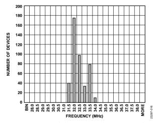
Figure 15. 32 MHz Clock Frequency Distribution, Untrimmed
