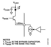
Figure 21. LED Driver Overvoltage Protection Circuit
