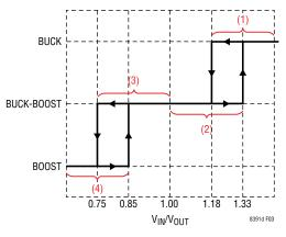
Figure 3. Operation Region vs V<sub>IN</sub>/V<sub>OUT</sub> Ratio
