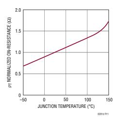
Figure 11. Normalized R<sub>DS(ON)</sub> vs Temperature
