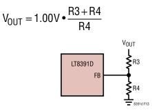
Figure 13. Feedback Resistor Connection
