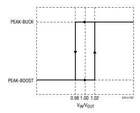
Figure 2. Current Mode vs  $V_{IN}/V_{OUT}$  Ratio
