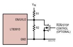
Figure 12. V<sub>IN</sub> Undervoltage Lockout (UVLO)
