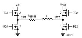
Figure 1. Simplified Diagram of the Power Switches
