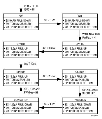
Figure 8. Start-Up and Fault Sequence
