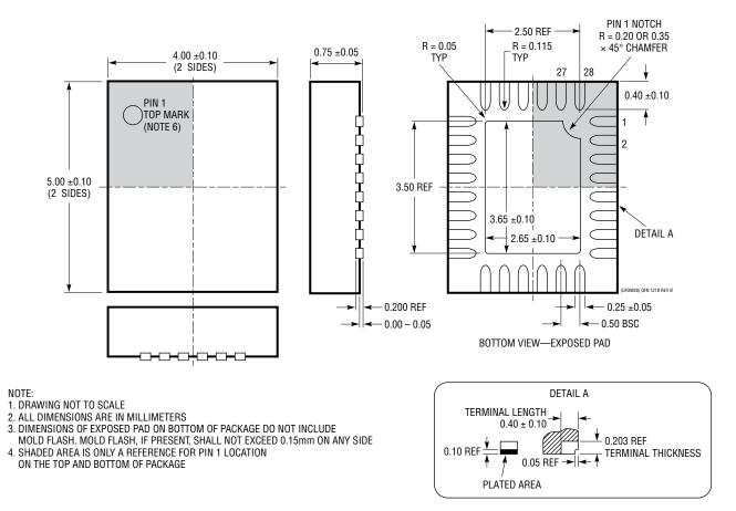
UFDM Package 28-Lead Plastic Side Wettable QFN (4mm × 5mm) (Reference LTC DWG # 05-08-1682 Rev Ø)
