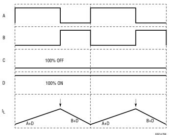
Figure 4. Peak-Buck in Buck Region ( $V_{IN} >> V_{OUT}$ )
