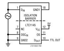
Figure 2. Common-Mode Rejection Test Circuit
