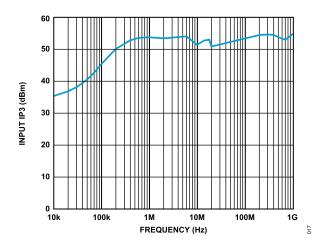
Figure 17. Input IP3 vs. Frequency, Low Frequency Detail
