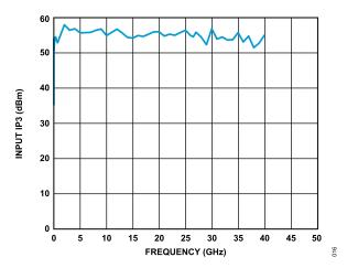
Figure 15. Input IP3 vs. Frequency
