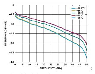
Figure 12. Insertion Loss vs. Frequency over Temperature
