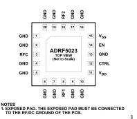
Figure 4. Pin Configuration (Top View)
