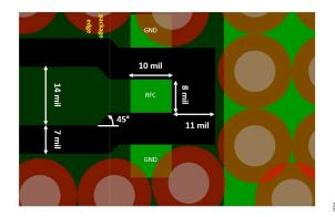
Figure 21. Recommended RF Pin Transitions
