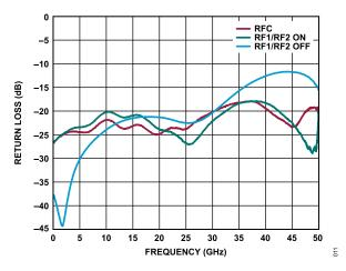
Figure 11. Return Loss vs. Frequency
