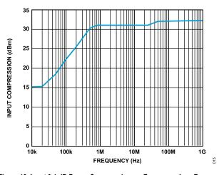
Figure 16. Input 0.1 dB Power Compression vs. Frequency, Low Frequency
