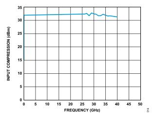
Figure 14. Input 0.1 dB Power Compression vs. Frequency
