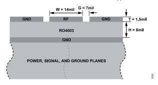
Figure 19. Example PCB Stack Up
