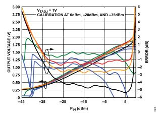
Figure 23. V<sub>RMS</sub> and Log Conformance Error vs. Input Level and Temperature at 8 GHz
