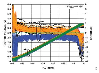
Figure 19. Distribution of Log Conformance Error with Respect to V<sub>RMS</sub> at 25°C vs. Input Level and Temperature at 2.14 GHz
