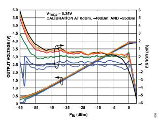
Figure 16. V<sub>RMS</sub> and Log Conformance Error vs. Input Level and Temperature at 2.14 GHz
