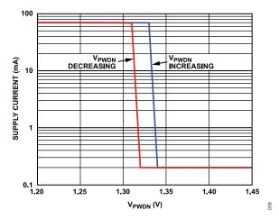
Figure 38. Supply Current vs. V<sub>PWDN</sub>
