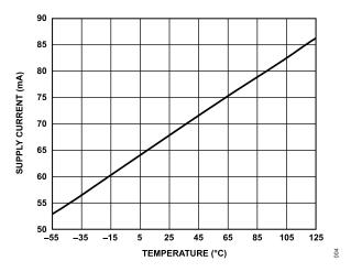
Figure 39. Supply Current vs. Temperature
