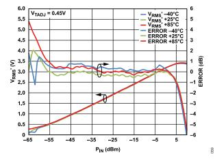
Figure 61. V<sub>RMS</sub>' and Log Conformance Error vs. Input Level and Temperature at 3500 MHz Using V<sub>TEMP</sub> Intercept Compensation
