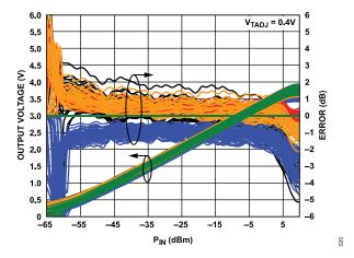
Figure 20. Distribution of Log Conformance Error with Respect to V<sub>RMS</sub> at 25°C vs. Input Level and Temperature at 2.6 GHz
