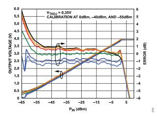
Figure 10.  $V_{\rm RMS}$  and Log Conformance Error vs. Input Level and Temperature at 700 MHz
