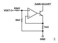
Figure 47. VSET Interface Simplified Schematic
