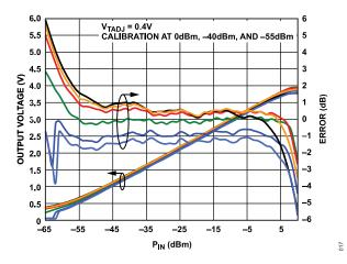
Figure 17.  $V_{\rm RMS}$  and Log Conformance Error vs. Input Level and Temperature at 2.6 GHz
