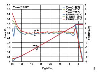
Figure 56. V<sub>RMS</sub>' and Log Conformance Error vs. Input Level and Temperature at 700 MHz Using V<sub>TEMP</sub> Intercept Compensation
