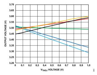
Figure 45. Effect of V<sub>TADJ</sub> at Various Temperatures, 2.14 GHz, 0 dBm
