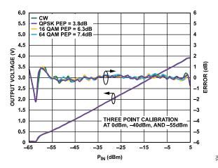
Figure 4. Error from CW Linear Reference vs. Signal Modulation (QPSK, 16 QAM, 64 QAM), Frequency = 900 MHz
