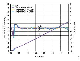
Figure 7. Error from CW Linear Reference vs. Signal Modulation (QPSK, 16 QAM, 64 QAM), Frequency = 2.14 GHz, Three Point Calibration at 0 dBm, -40 dBm, and -55 dBm
