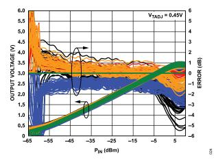
Figure 24. Distribution of Log Conformance Error with Respect to V<sub>RMS</sub> at 25°C vs. Input Level and Temperature at 3.5 GHz
