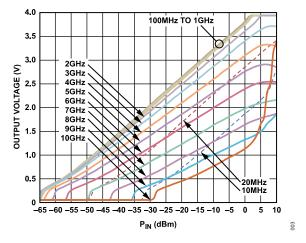
Figure 3. Typical V<sub>RMS</sub> vs. Input Power (dBm) vs. Frequency (10 MHz to 10 GHz) at 25°C
