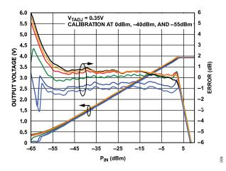
Figure 9. V<sub>RMS</sub> and Log Conformance Error vs. Input Level and Temperature at 100 MHz
