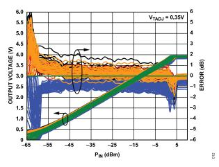
Figure 12. Distribution of Log Conformance Error with Respect to V<sub>RMS</sub> at 25°C vs. Input Level and Temperature at 100 MHz
