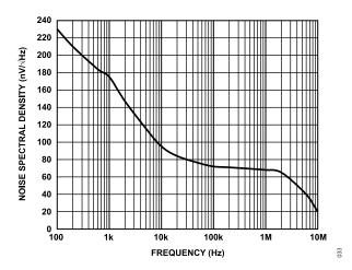
Figure 33. Noise Spectral Density of  $V_{RMS}$ ,  $P_{IN}$  = -10 dBm, -35 dBm, and -60 dBm (No Change in NSD vs.  $P_{IN}$ )
