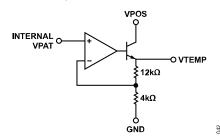
Figure 43. TEMP Interface Simplified Schematic
