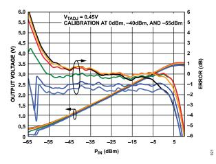
Figure 21.  $V_{\rm RMS}$  and Log Conformance Error vs. Input Level and Temperature at 3.5 GHz
