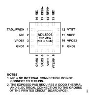
Figure 2. Pin Configuration
