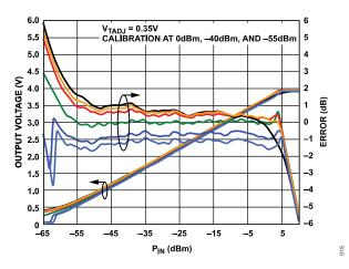
Figure 15. V<sub>RMS</sub> and Log Conformance Error vs. Input Level and Temperature at 1.9 GHz
