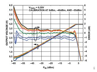
Figure 11. V<sub>RMS</sub> and Log Conformance Error vs. Input Level and Temperature at 900 MHz
