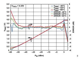
Figure 58. V<sub>RMS</sub>' and Log Conformance Error vs. Input Level and Temperature at 1900 MHz Using V<sub>TEMP</sub> Intercept Compensation
