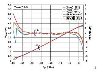
Figure 60.  $V_{\rm RMS}$ ' and Log Conformance Error vs. Input Level and Temperature at 2600 MHz Using  $V_{\rm TEMP}$  Intercept Compensation
