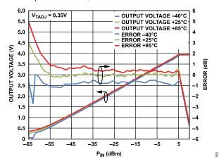
Figure 54. 2.14 GHz V<sub>RMS</sub> and Log Conformance Error at +25°C, -40°C, and +85°C Using Three-Point Calibration at 0 dBm, -40 dBm, and -55 dBm
