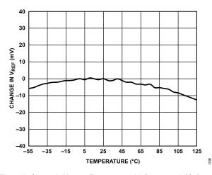
Figure 36. Change in  $V_{REF}$  vs. Temperature with Respect to 25°C,  $P_{IN}$  = -40 dRm
