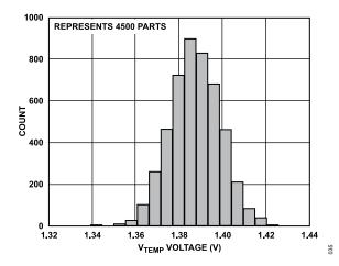
Figure 35. Distribution of V<sub>TEMP</sub> at 25°C, No RF Input
