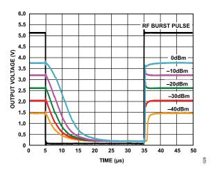
Figure 29. Output Response to RF Burst Input, Carrier Frequency = 2.14 GHz,  $C_{RMS}$  = 1 nF
