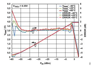
Figure 55. V<sub>RMS</sub>' and Log Conformance Error vs. Input Level and Temperature at 100 MHz Using V<sub>TEMP</sub> Intercept Compensation
