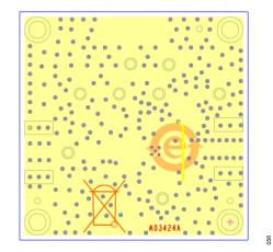
Figure 65. ADL5906 Evaluation Board Layout, Bottom Side
