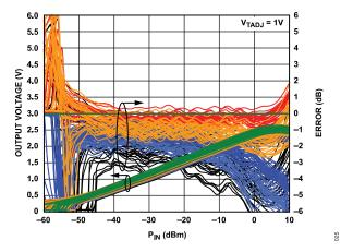
Figure 25. Distribution of Log Conformance Error with Respect to V<sub>RMS</sub> at 25°C vs. Input Level and Temperature at 5.8 GHz
