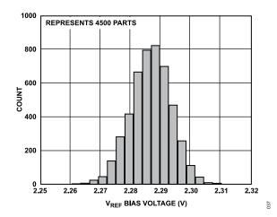
Figure 37. Distribution of V<sub>REF</sub> at 25°C, No RF Input
