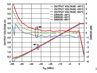
Figure 53. 2.14 GHz V<sub>RMS</sub> and Log Conformance Error at +25°C, -40°C, and +85°C Using Two-Point Calibration at 0 dBm and -40 dBm
