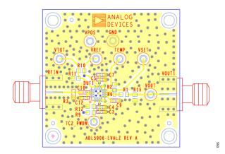
Figure 64. ADL5906 Evaluation Board Layout, Top Side
