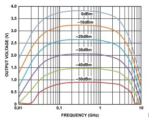
Figure 6. Typical V<sub>RMS</sub> vs. Frequency for Six RF Input Levels
