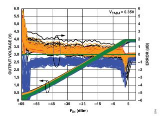
Figure 14. Distribution of Log Conformance Error with Respect to V<sub>RMS</sub> at 25°C vs. Input Level and Temperature at 900 MHz
