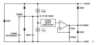
Figure 48. VRMS Interface Simplified Schematic
