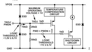
Figure 46. TADJ/PWDN Interface Simplified Schematic
