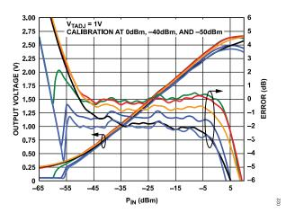
Figure 22.  $V_{\rm RMS}$  and Log Conformance Error vs. Input Level and Temperature at 5.8 GHz
