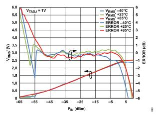
Figure 62.  $V_{\rm RMS}$ ' and Log Conformance Error vs. Input Level and Temperature at 5800 MHz Using  $V_{\rm TEMP}$  Intercept Compensation
