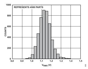
Figure 28. Distribution of  $V_{RMS}$ ,  $P_{IN} = -45$  dBm, 900 MHz
