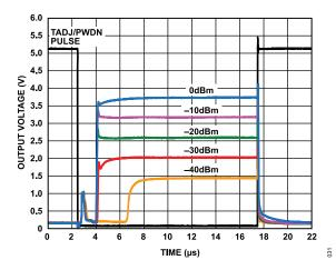
Figure 31. Output Response Using Power-Down Mode for Various RF Input Levels, Carrier Frequency = 2.14 GHz, C<sub>RMS</sub> = 1 nF
