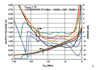
Figure 26. V<sub>RMS</sub> and Log Conformance Error vs. Input Level and Temperature at 10 GHz
