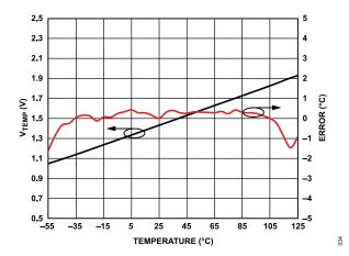
Figure 34. V<sub>TEMP</sub> and Linearity Error with Respect to Straight Line vs.
