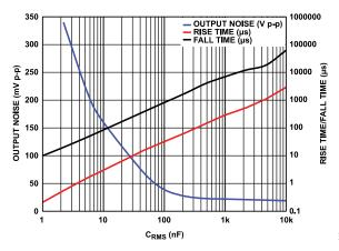
Figure 50 also shows how the response time is affected by the value of  $C_{RMS}$ . To measure this, an RF burst at 2.14 GHz at 0 dBm was applied to the ADL5906. The 10% to 90% rise time and 90% to 10% fall time were then measured.
