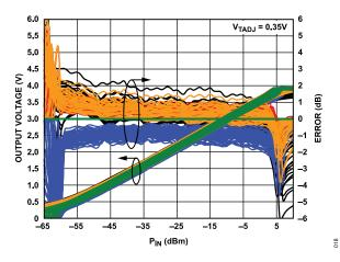
Figure 18. Distribution of Log Conformance Error with Respect to V<sub>RMS</sub> at 25°C vs. Input Level and Temperature at 1.9 GHz
