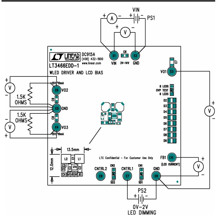
Figure 1. Test Connection Diagram
