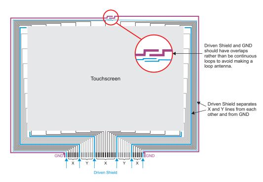
NOTE: Sample touchscreen for illustrative purposes only. The number of X/Y lines available on any given device might differ from that shown here. Similarly, the routing of the X/Y lines shown should not be taken as indicative of any preferred layout and the user's layout may vary.
