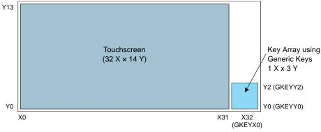
Note: Generic Key X line (GKEYX0) is logically situated at X32 and Generic Key Y lines (GKEYY0 to GKEYY2) are logically situated at Y0 to Y2.
