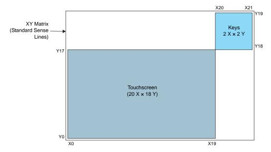
FIGURE 4-2: EXAMPLE LAYOUT – TOUCHSCREEN WITH GENERIC KEYS
