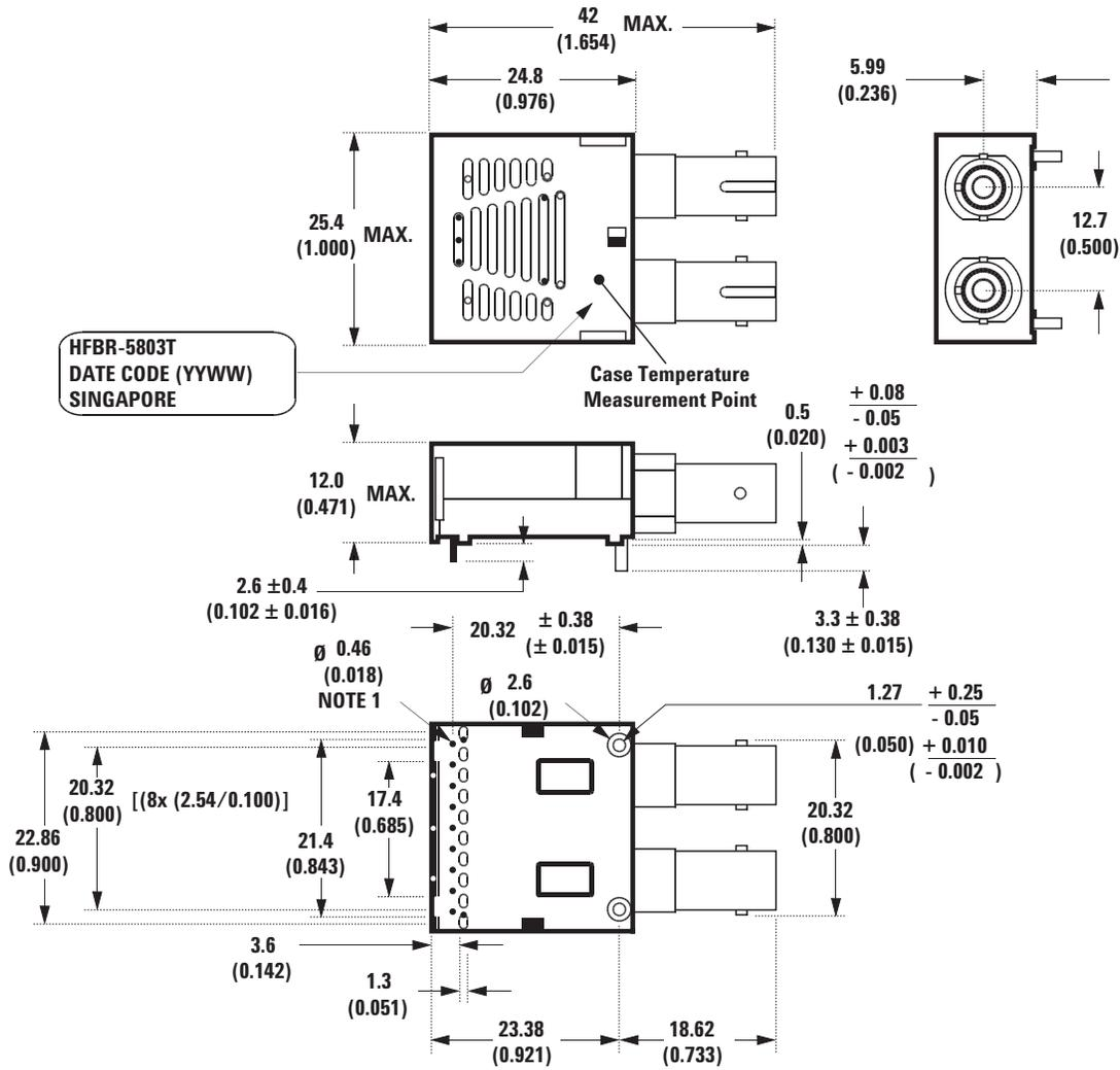
NOTE 1: PHOSPHOR BRONZE IS THE BASE MATERIAL FOR THE POSTS & PINS WITH TIN LEAD OVER NICKEL PLATING.
