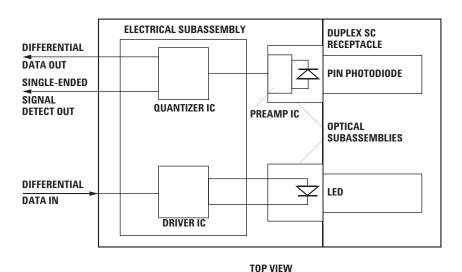
**Figure 1. SC Connector Block Diagram**
