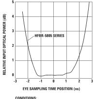
CONDITIONS:  $1.\,T_A = +25^\circ \,C$   $2.\,V_{CC} = 3.3\,V \text{ to 5 V dc}$   $3.\,INPUT OPTICAL RISE/FALL TIMES = 1.0/2.1 \text{ ns.}$   $4.\,INPUT OPTICAL POWER IS NORMALIZED TO CENTER OF DATA SYMBOL.$   $5.\,NOTE 16 \text{ AND } 17\,\text{APPLY.}$
