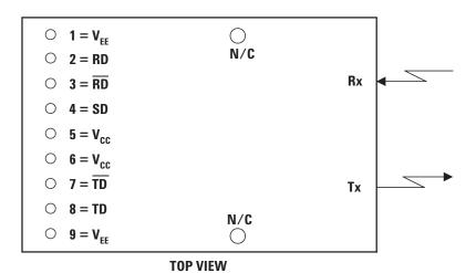
Figure 3. Pin Out Diagram.
