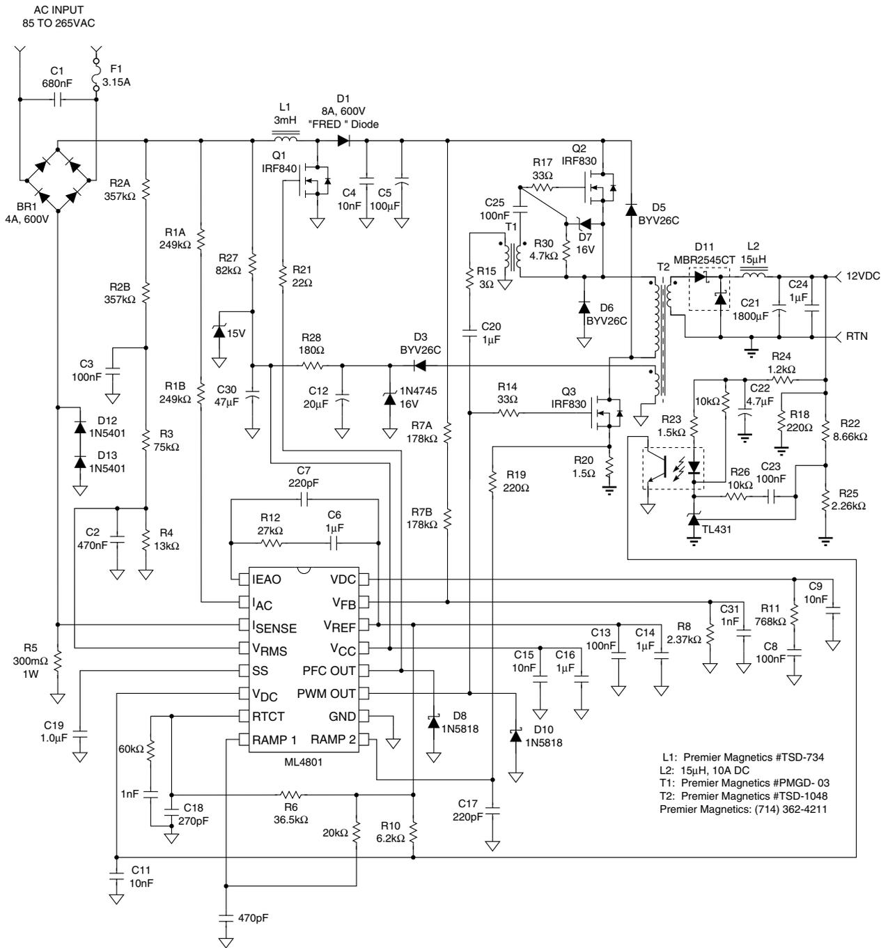
Figure 9. 100W Power Factor Corrected Power Supply
