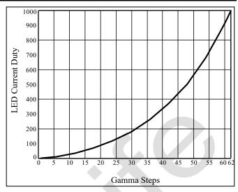
Figure 20 Gamma Correction (63 Steps)
