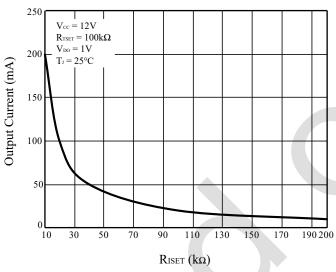
Figure 4 Output Current vs. R<sub>ISET</sub>
