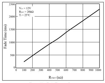
Figure 19 Fade Time vs. R<sub>TSET</sub>
