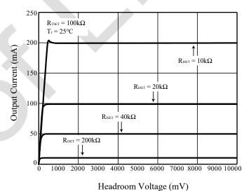
Figure 5 Output Current vs. Headroom Voltage
