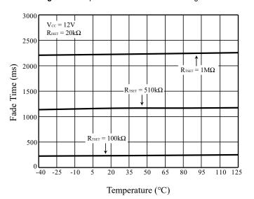
Figure 7 Fade Time vs. Temperature
