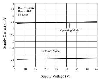
Figure 2 Supply Current vs. Supply Voltage
