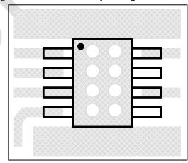
Figure 22 Board Via Layout For Thermal Dissipation
