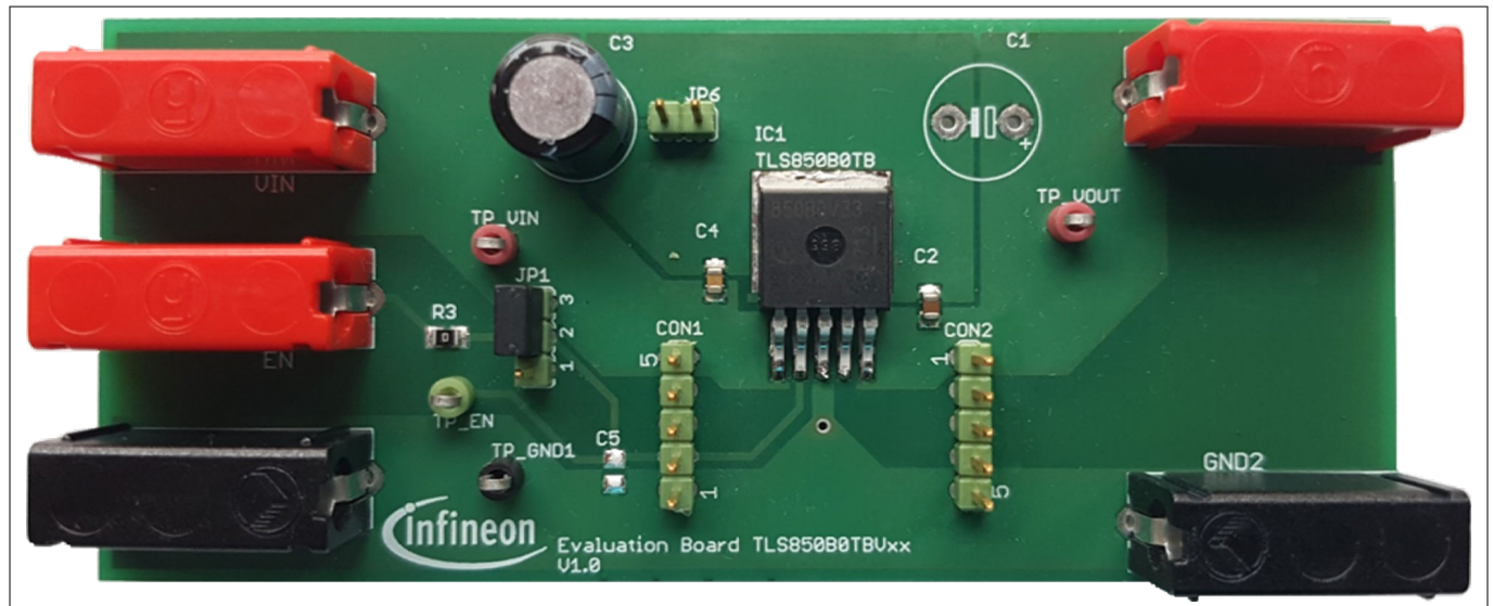
Figure 2 OPTIREG™ linear voltage regulator TLS850B0TBVxx demoboard
