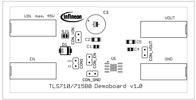
Figure 6 Top Layer components of TLS710/715B0 Demoboard
