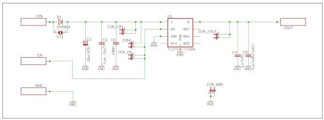
Figure 3 Schematic of TLS710/715B0 Demoboard
