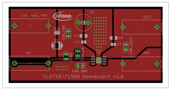
Figure 4 Top Layer of TLS710/715B0 Demoboard
