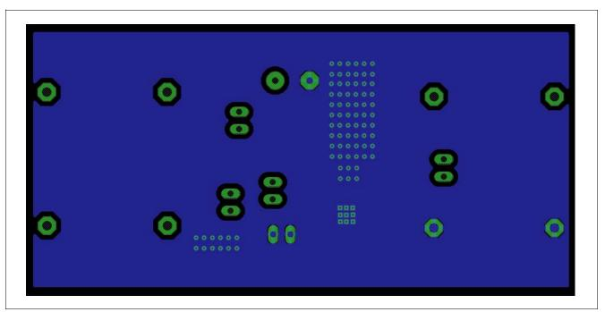
Figure 5 Bottom Layer of TLS710/715B0 Demoboard
