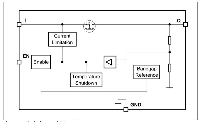
Figure 1 Block Diagram of TLS710/715B0
