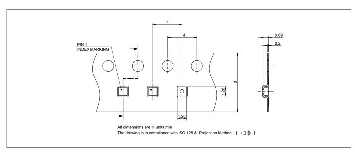
Figure 6: Carrier Tape (top and side views)
