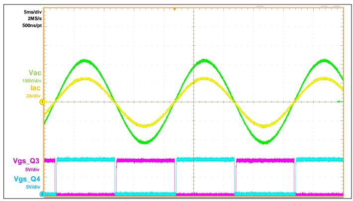
Figure 12 Steady-state waveforms of active-bridge low-side complementary driving signals (magenta and light blue lines), input current and voltage (yellow and green lines) and PFC output voltage (light blue line) at 230 V<sub>AC</sub>
