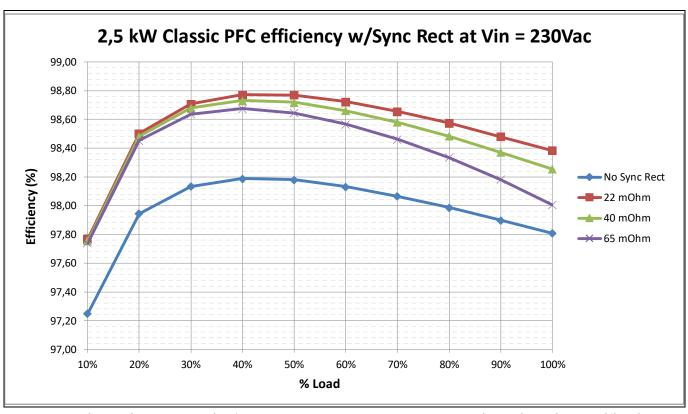
Figure 16 Simulation results with (22 m $\Omega$ , 40 m $\Omega$ , 65 m $\Omega$ ) and without active-bridge line rectification at high-line
