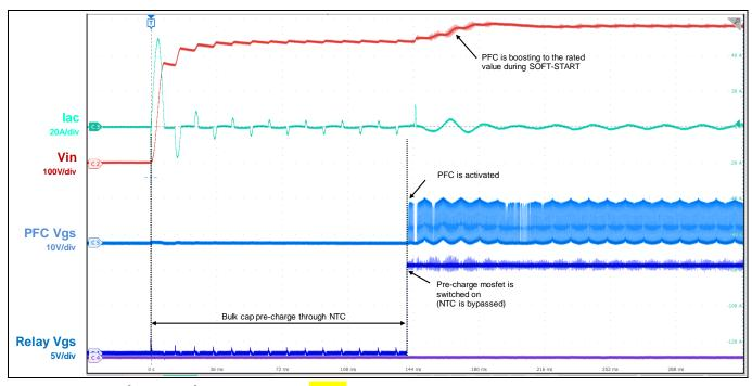
Figure 29 Pre-charge and PFC start-up at 250 V<sub>AC</sub>
