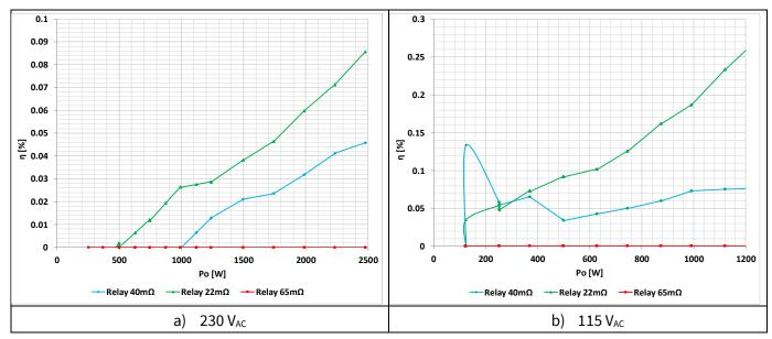
Figure 21 Delta efficiency test result of EVAL\_2K4W\_ACT\_BRD\_S7: comparison of relay MOSFETs with different R<sub>DS ON</sub>
