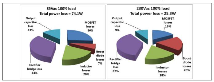
Figure 13 Power dissipation of power devices with a 1000 W PFC circuit at 85 V<sub>AC</sub> and 230 V<sub>AC</sub>
