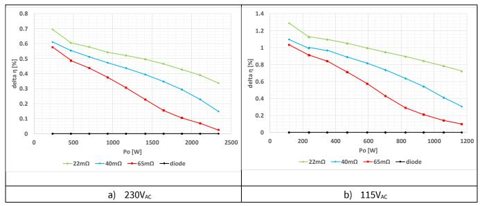
Figure 20 Delta efficiency test result of EVAL\_2K4W\_ACT\_BRD\_S7: comparison between passive and active bridge at different R<sub>DS.ON</sub>
