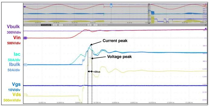
Figure 33 Zoom: voltage drop of 20 ms at 1800 W
