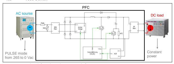
Figure 31 Test-bench for voltage drop-out emulation
