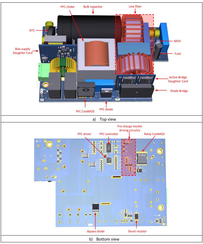
Figure 5 Placement of the different components in the 2400 W active-bridge CCM PFC with Infineon 600 V CoolMOS™ S7 MOSFET
