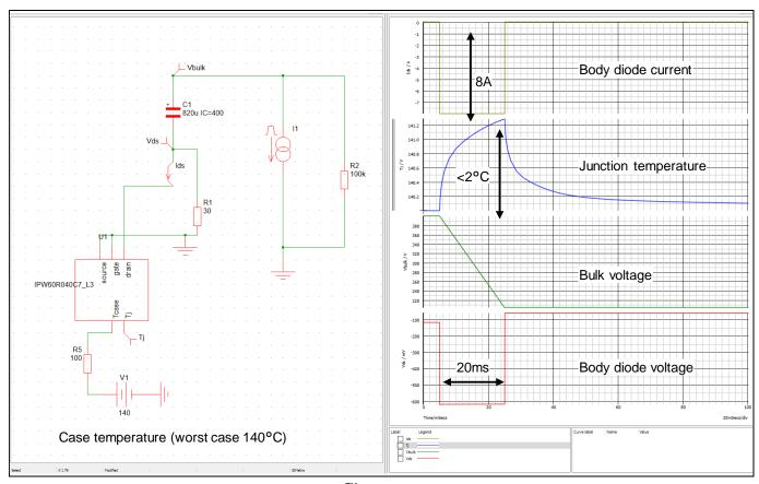
Simulation in case of relay CoolMOS<sup>™</sup> body diode conducting during voltage drop-out Figure 35
