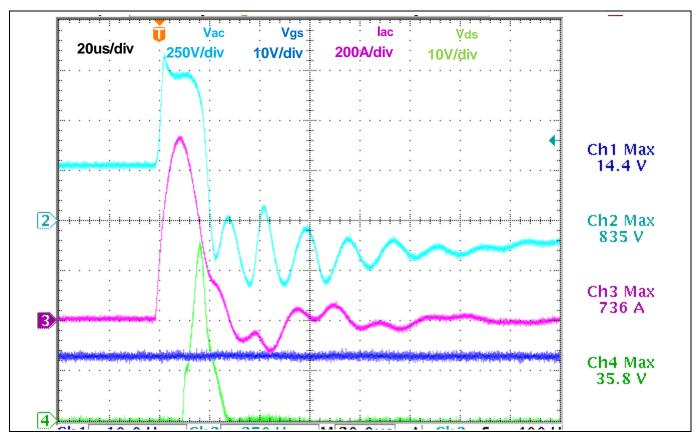
Figure 40 Experimental results of 2 kV surge without active bridge
