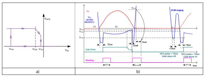
Behavior of IR11688S: a) input comparator thresholds and b) example of waveforms Figure 11
