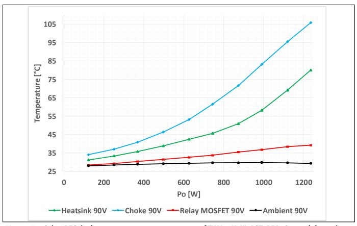
Figure 25 Other PFC devices temperature measurements of EVAL\_2K4W\_ACT\_BRD\_S7 at minimum low-line
