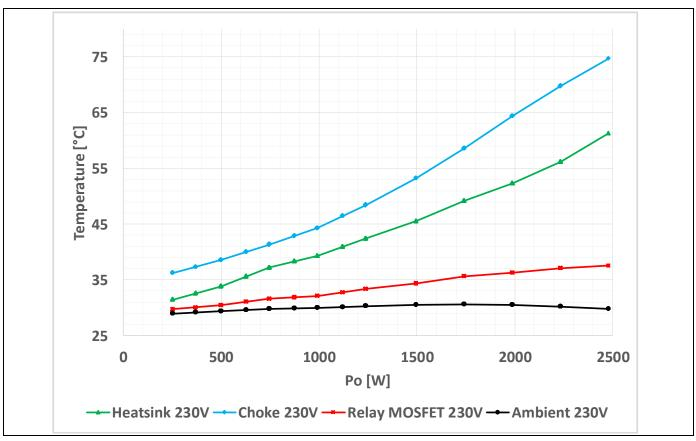
Figure 24 Other PFC devices temperature measurements of EVAL\_2K4W\_ACT\_BRD\_S7 at nominal high-line
