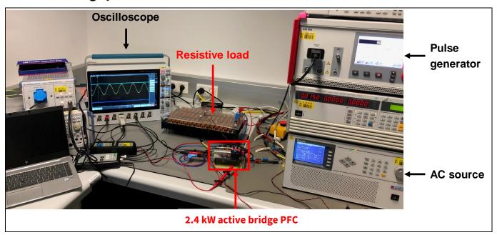
Figure 37 Surge pulse test bench
