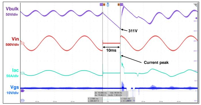
Figure 32 Voltage drop of 20 ms at 1800 W
