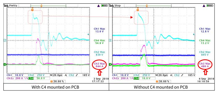
Figure 43 2 kV surge pulse BULK current
