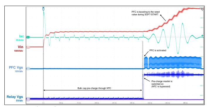
Figure 30 Pre-charge and PFC start-up at 120 V<sub>AC</sub>
