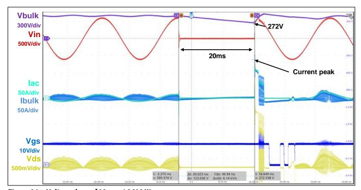
Figure 34 Voltage drop of 10 ms at 2400 W
