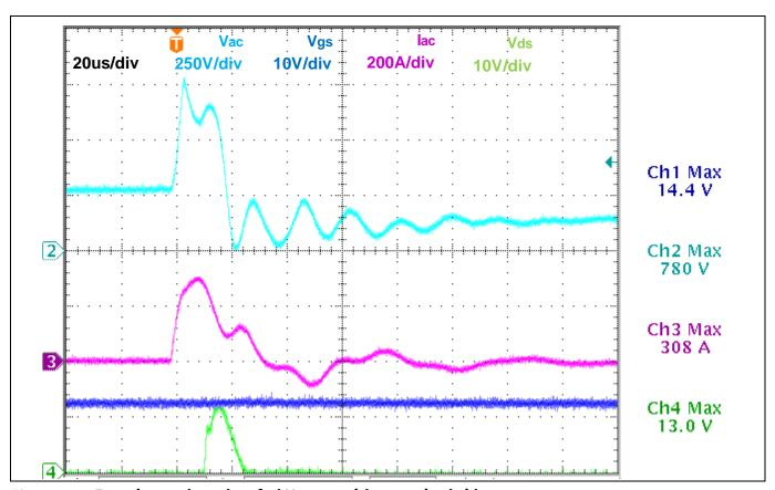
Figure 39 Experimental results of 1 kV surge without active bridge
