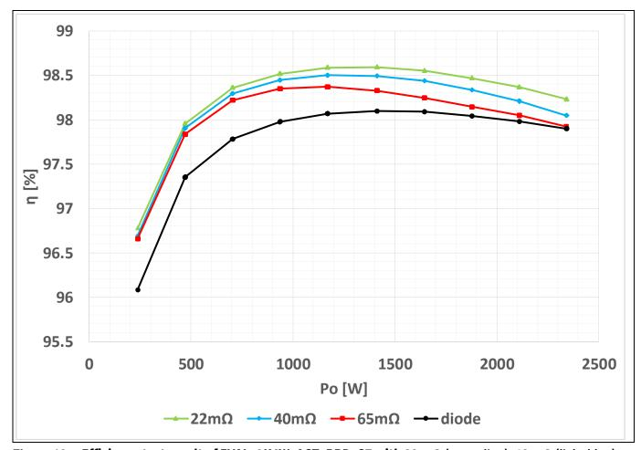
Figure 18 Efficiency test result of EVAL\_2K4W\_ACT\_BRD\_S7 with 22 m $\Omega$  (green line), 40 m $\Omega$  (light blue), 65 m $\Omega$  (red) active-bridge line rectification and with only the diode bridge (black) at 230 V<sub>AC</sub>
