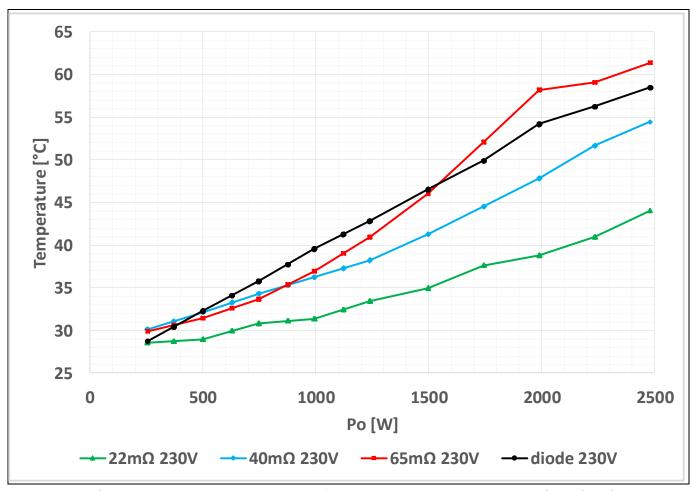
Bridge temperature measurements of EVAL\_2K4W\_ACT\_BRD\_S7 at nominal high-line Figure 22
