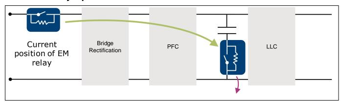
Inrush current device from AC-side to DC-link side
