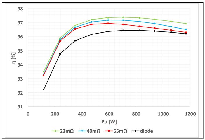
Figure 19 Efficiency test result of EVAL\_2K4W\_ACT\_BRD\_S7 with 22 m $\Omega$ , 40 m $\Omega$ , 65 m $\Omega$  full-wave active-bridge line rectification and without active bridge (passive) at 115  $V_{AC}$
