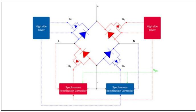
Figure 9 Second approach based on the SR controller
