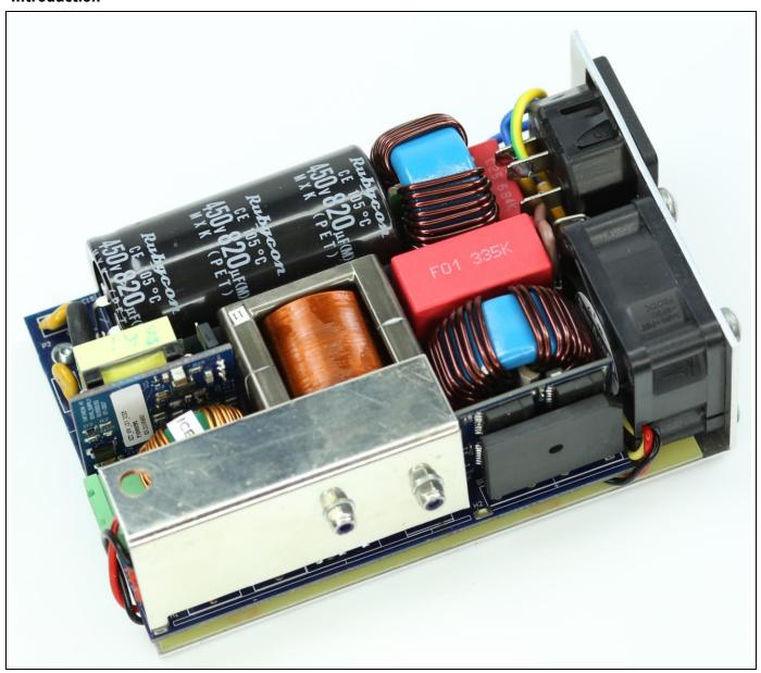
2400 W active-bridge CCM PFC based on 600 V CoolMOS™ S7 Figure 1
