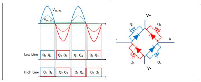
Figure 7 Control concept of the active-bridge line rectification
