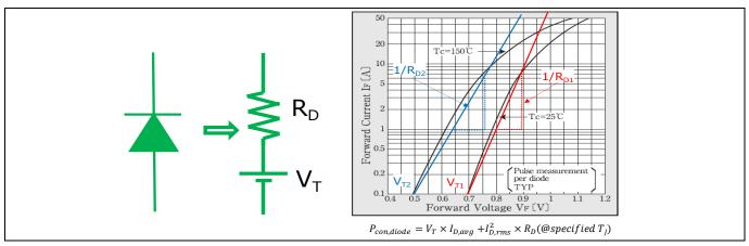
Figure 14 The equivalent circuit and the conduction loss of the diode
