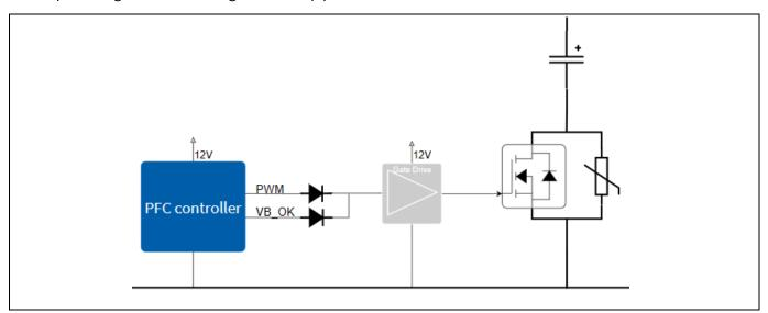
Figure 28 Control network of the pre-charge MOSFET
