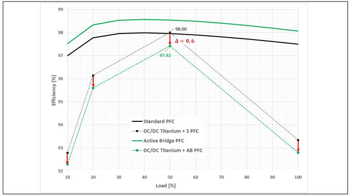
Reduction of DC-DC efficiency requirements for a PLUS Titanium design thanks to the active Figure 2 bridge (at 230 V<sub>AC</sub>)
