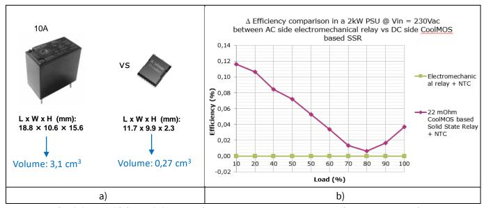
Figure 27 Size (a) and efficiency (b) comparison between standard mechanical relay at AC-side and CoolMOS<sup>™</sup>-based solution at DC-side
