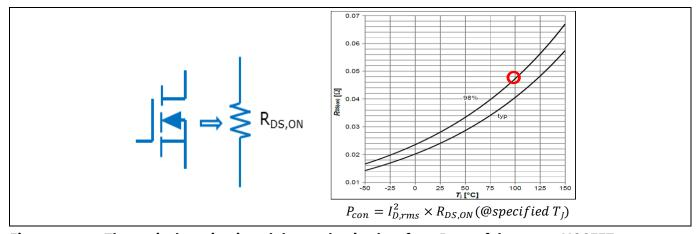
Figure 15 The equivalent circuit and the conduction loss from R<sub>DS,ON</sub> of the power MOSFET
