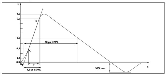
Figure 36 Surge voltage waveform according to IEC 61000-4-5
