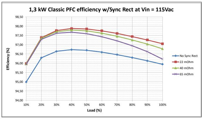
Figure 17 Simulation results with (22 m $\Omega$ , 40 m $\Omega$ , 65 m $\Omega$ ) and without active-bridge line rectification at low-line
