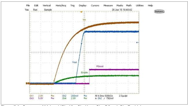
Figure 7-6 Startup at 20A Load (Ch<sub>1</sub>:Vin, Ch<sub>2</sub>:Vout, Ch<sub>3</sub>: PGood, Ch<sub>4</sub>:Enable)
