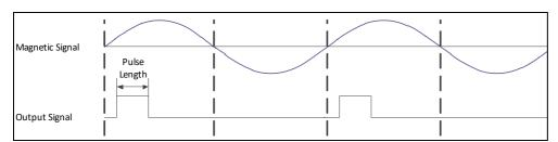
Figure 2-2 Output Pulses on magnetic rising edge
