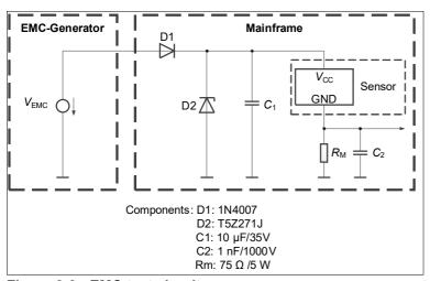
Figure 3-3 EMC test circuit
