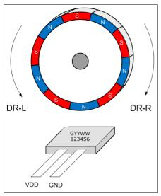
Figure 2-3 Definition of Rotation Direction
