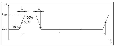
Figure 3-2 Definition of Rise and Fall Time
