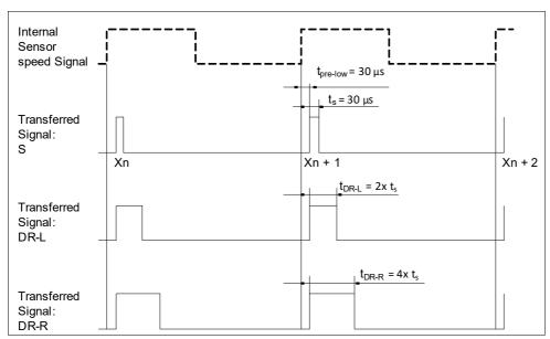
Figure 3-1 Definition of PWM Current Interface
