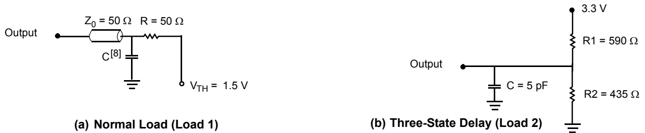
Figure 3. AC Test Load and Waveforms
