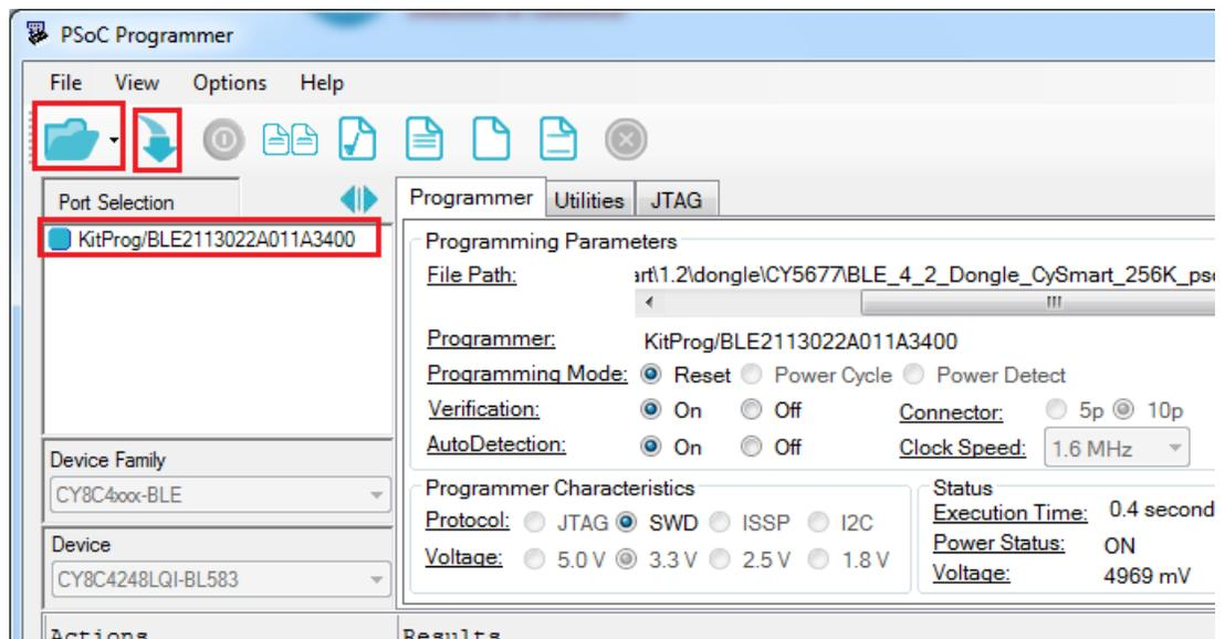
4. Ensure the other settings match as shown in [Figure 3-16](#). Click the **Program** button to start programming. The status bar at the bottom of the PSoC Programmer window will show the programming status and the result (Pass/Fail).
