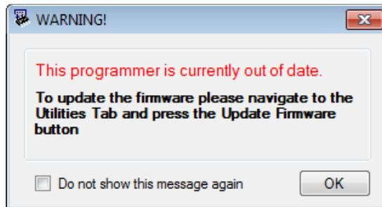
To update the KitProg, go to the **Utilities** tab on PSoC Programmer and click **Upgrade Firmware**, as shown in [Figure 3-19](#).
