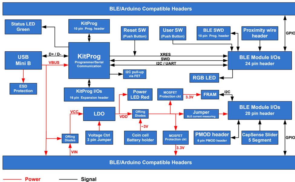
The BLE Pioneer Baseboard acts as the baseboard for the PSoC 4 BLE Module. The BLE Pioneer Baseboard contains a PSoC 5LP device, that has KitProg firmware, used as an onboard programmer or debugger, and for the USB-Serial interface.
