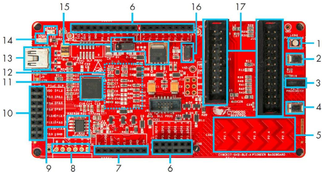
Figure 1-3 shows a markup of the onboard components of the PSoC 4 BLE module. See [BLE Modules and BLE Dongles Compatible with the BLE Pioneer Kit](#) on page 115 for more details. Figure 1-4 shows the BLE Dongle board blocks.
