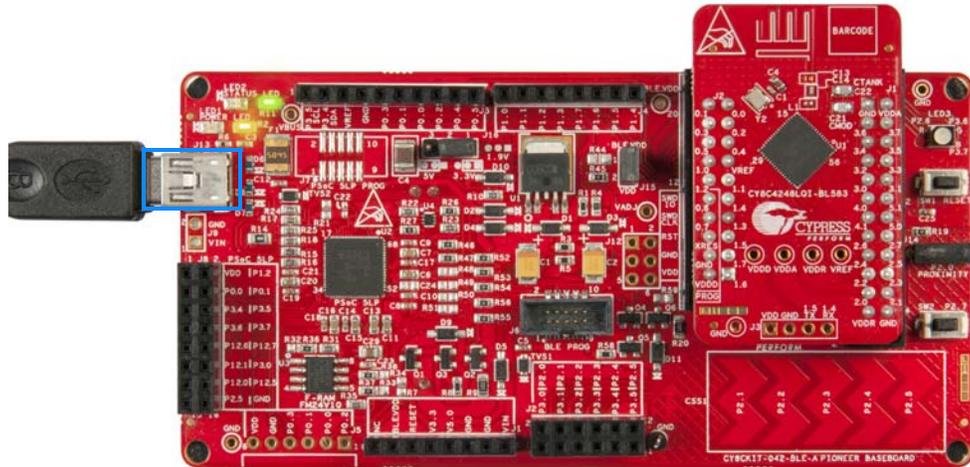
Figure 3-8. Connect Dongle to PC
