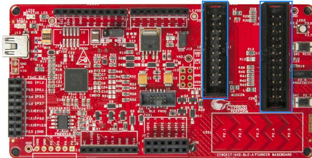
To remove the PSoC 4 BLE Module from the BLE Pioneer Kit, hold the BLE Pioneer Kit in one hand and the module in the other, as shown in Figure 3-6, and pull it out using a rocking motion.
