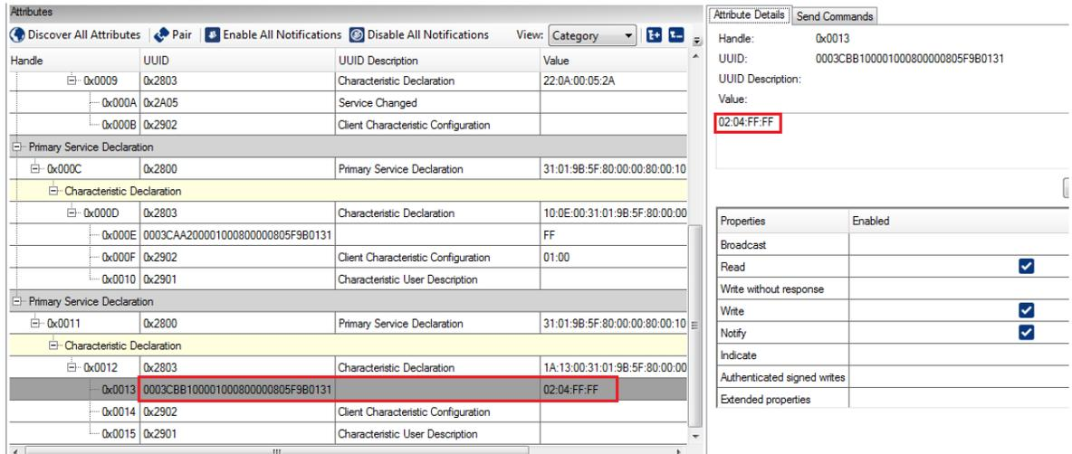
The screenshot shows the Bluetooth LE Explorer interface. The main table lists characteristics, with 0x0013 selected and highlighted in red. The 'Value' field for this characteristic is set to 02:04:FF:FF. The right-hand pane shows the 'Attribute Details' for 0x0013, with the 'Value' field also containing 02:04:FF:FF. The 'Properties' section on the right shows that 'Write' is checked.
