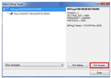
8. After the device is acquired, it is shown in a tree structure below the **KitProg2/<serial number>**. Click the **Connect** button and then click **OK** to exit the window and start programming, as shown in Figure 4-5.
