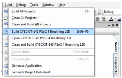
4. If there are no errors during build, program the firmware into the kit by choosing **Debug** > **Program** or press **[Ctrl] [F5]**, as shown in Figure 3-4. This programs the target PSoC 4200DS device on the PSoC 4200DS Prototyping kit, and the kit is ready to use.
