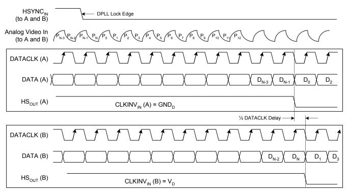
FIGURE 9. ALTERNATE PIXEL SAMPLING (24 BIT MODE)
