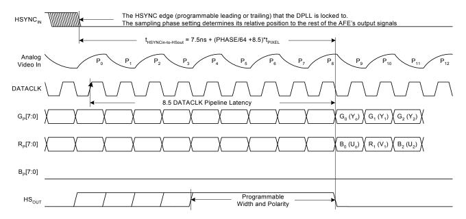
FIGURE 4. 24 BIT 4:2:2 OUTPUT MODE (FOR YUV SIGNALS)
