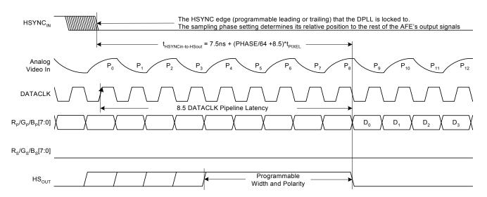
FIGURE 3. 24 BIT OUTPUT MODE
