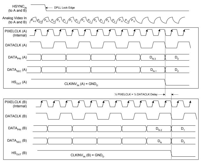
FIGURE 10. ALTERNATE PIXEL SAMPLING (48 BIT MODE)
