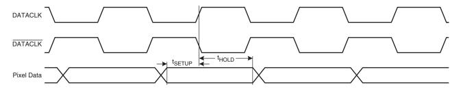
FIGURE 2. DATA OUTPUT SETUP AND HOLD TIMING
