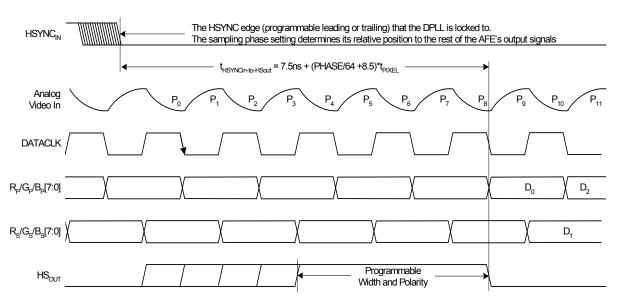
FIGURE 6. 48 BIT OUTPUT MODE, INTERLEAVED TIMING
