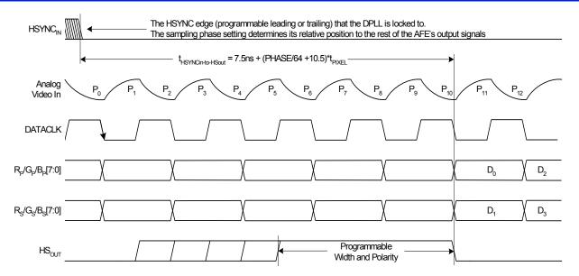
FIGURE 5. 48 BIT OUTPUT MODE
