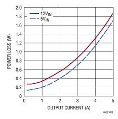
Figure 9. 1.5V Output Power Loss
