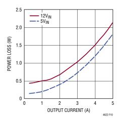
Figure 10. 2.5V Output Power Loss
