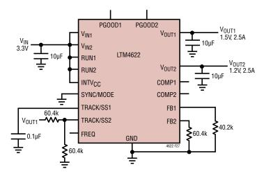
Figure 27.  $3.3V_{IN}$ , 1.5V and 1.2V Output at 2.5A Design with Output Coincident Tracking
