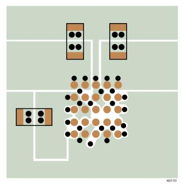
Figure 23. Recommended PCB Layout
