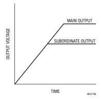
Figure 6. Output Coincident Tracking Waveform
