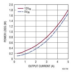
Figure 8. 1V Output Power Loss
