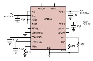
Figure 26.  $\,$  8V  $_{\mbox{\footnotesize IN}}$  to 20V  $_{\mbox{\footnotesize IN}},\,3.3$ V and 5V Output at 2.5A with 2MHz Switching Frequency
