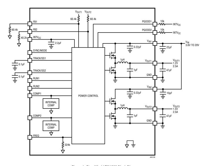
Figure 1. Simplified LTM4622 Block Diagram
