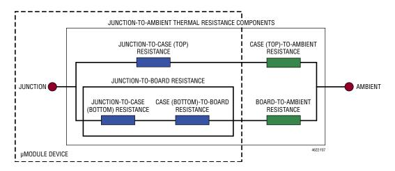
Figure 7. Graphical Representation of JESD 51-12 Thermal Coefficients
