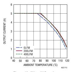
Figure 13. 5V to 1V Derating Curve, No Heat Sink
