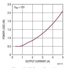
Figure 12. 5V Output Power Loss
