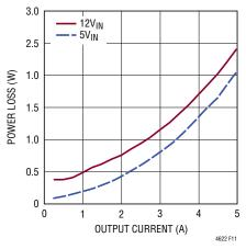
Figure 11. 3.3V Output Power Loss
