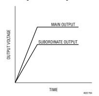
Figure 4. Output Ratiometric Tracking Waveform
