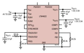
Figure 5. Example Schematic of Ratiometric Output Voltage Tracking
