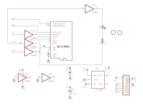
For the level shifter we use the  $\underline{\text{CD74HC4050}}$  () which has a typical propagation delay of ~10ns
