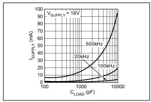
FIGURE 2-7: Supply Current vs. Capacitive Load.
