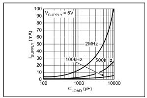
FIGURE 2-11: Supply Current vs. Capacitive Load.
