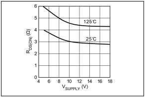
FIGURE 2-18: Output Resistance (Output Low) vs. Supply Voltage.
