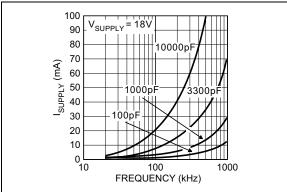
FIGURE 2-8: Supply Current vs. Frequency.
