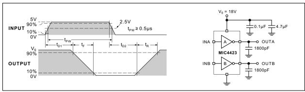
FIGURE 1-1: Inverting Driver Switching Time.
