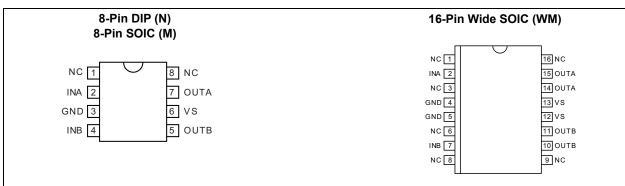
Note: WM Package: Duplicate GND, VS, OUTA, and OUTB pins must be externally connected together.
