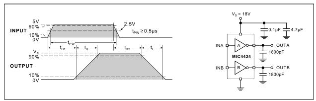
FIGURE 1-2: Non-Inverting Driver Switching Time.
