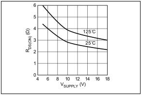
**FIGURE 2-17:** Output Resistance (Output High) vs. Supply Voltage.
