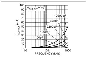
FIGURE 2-12: Supply Current vs. Frequency.
