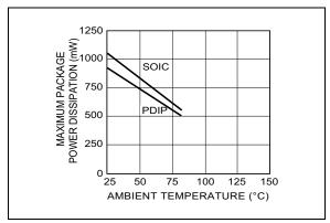
**FIGURE 4-2:** Power Dissipation vs. Ambient Temperature.
