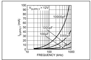
**FIGURE 2-10:** Supply Current vs. Frequency.
