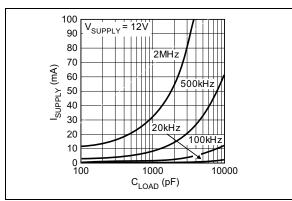
FIGURE 2-9: Supply Current vs. Capacitive Load.
