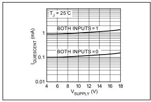
FIGURE 2-15: vs. Voltage.
