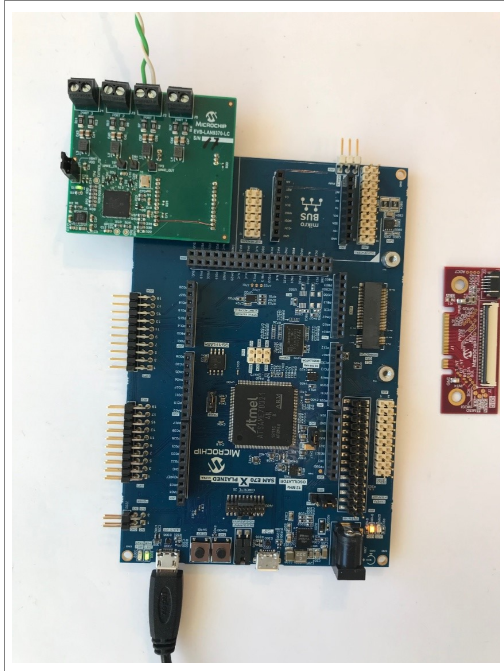
FIGURE 2-1: EVB-LAN9370 CONNECTION TO SAM E70
