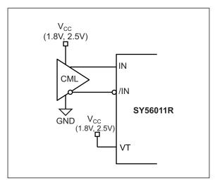
**FIGURE 7-2:** CML Interface  $50\Omega$  to  $V_{CC}$  (DC-Coupled, 1.8V, 2.5V).
