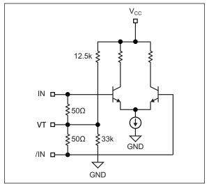
**FIGURE 6-1:** Simplified Differential Input Buffer.
