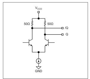
FIGURE 6-2: Simplified CML Output Buffer.
