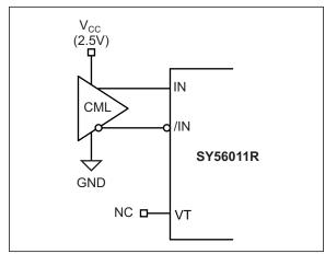
**FIGURE 7-1:** CML Interface  $100\Omega$  Differential (DC-Coupled, 2.5V).
