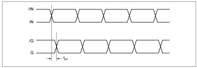
FIGURE 4-1: Propagation Delay.
