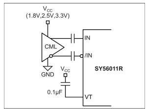
FIGURE 7-3: CML Interface (AC-Coupled).
