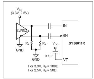
FIGURE 7-4: LVPECL Interface (AC-Coupled).
