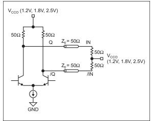
FIGURE 8-1: 1.2V, 1.8V, 2.5V CML DC-Coupled Termination.
