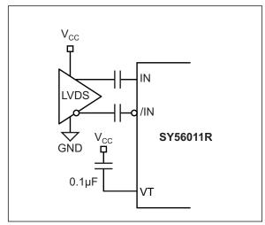
FIGURE 7-5: LVDS Interface (AC Coupled).
