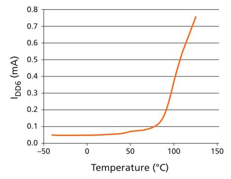
Figure 3: V<sub>DD2</sub> Typical Self-Refresh Current vs. Temperature
