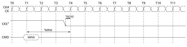
Note: 1. CKE can be registered LOW <sup>t</sup>MRW after the clock on which the MRW command is registered.
