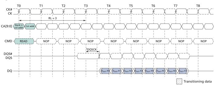
Figure 15: Burst READ – RL = 3, BL = 8, <sup>t</sup>DQSCK < <sup>t</sup>CK
