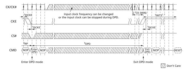
Figure 62: Deep Power-Down Entry and Exit Timing
