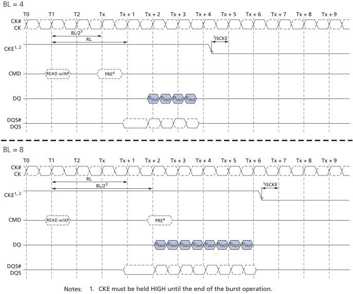
2. CKE can be registered LOW at (RL + RU(<sup>t</sup>DQSCK/<sup>t</sup>CK)+ BL/2 + 1) clock cycles after the clock on which the READ command is registered.
