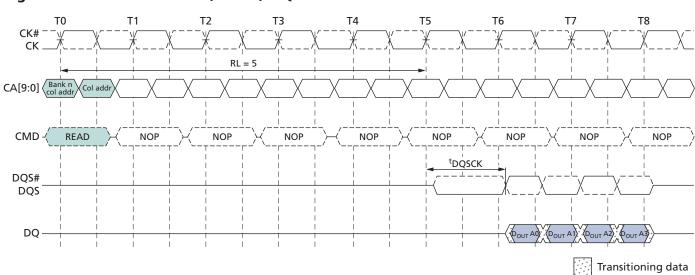
Figure 14: Burst READ – RL = 5, BL = 4, <sup>t</sup>DQSCK > <sup>t</sup>CK
