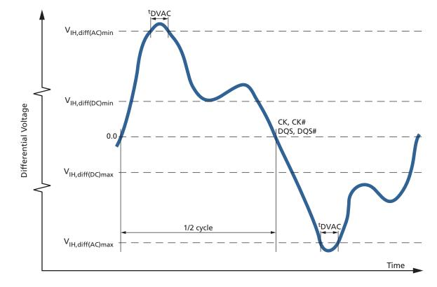
Figure 67: Differential AC Swing Time and <sup>t</sup>DVAC
