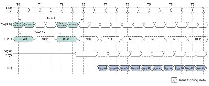
Figure 21: READ Burst Interrupt Example – RL = 3, BL = 8, <sup>t</sup>CCD = 2
