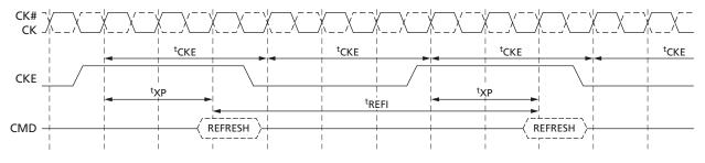
Note: 1. The pattern shown can repeat over an extended period of time. With this pattern, all AC and DC timing and voltage specifications with temperature and voltage drift are ensured.
