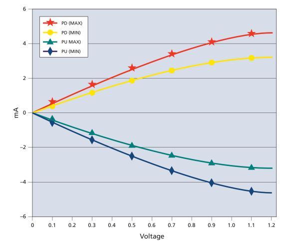
Figure 77: Output Impedance = 240 Ohms, I-V Curves After Calibration
