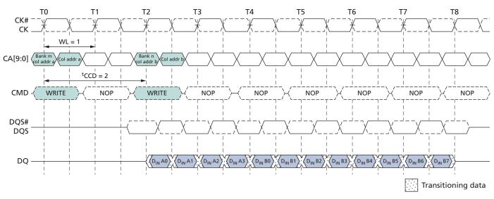
Figure 26: WRITE Burst Interrupt Timing – WL = 1, BL = 8, <sup>t</sup>CCD = 2
