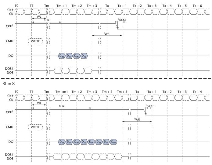
Note: 1. CKE can be registered LOW at (WL + 1 + BL/2 + RU(<sup>t</sup>WR/<sup>t</sup>CK)) clock cycles after the clock on which the WRITE command is registered.
