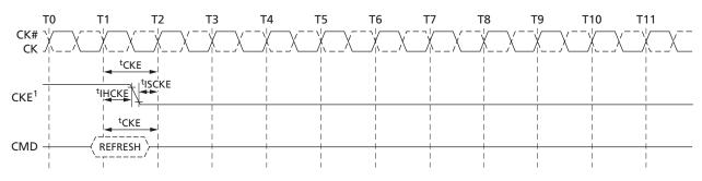
Note: 1. CKE can go LOW <sup>t</sup>IHCKE after the clock on which the REFRESH command is registered.
