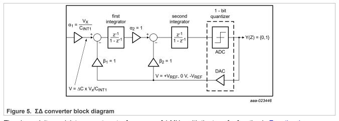
The sigma delta modulator operates at a frequency of 1 MHz, with the transfer function in Equation 1.
