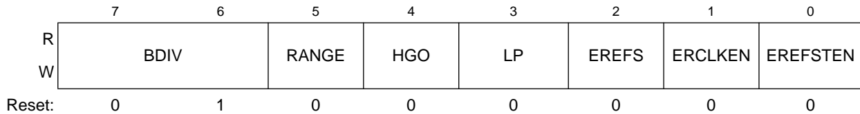
Figure 8-4. MCG Control Register 2 (MCGC2)
