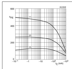
**TR2 (PNP)**  $V_{CE} = -2 \text{ V}.$
