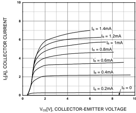
Figure 1. Static Characteristic
