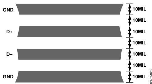
Figure 20. Arrangement of Signal Tracks
