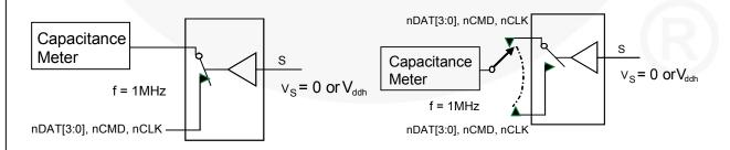
Figure 14. Channel On Capacitance
