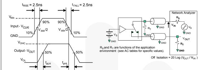
Figure 11. CLK Propagation Delay Waveforms
