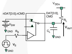
$R_L$ ,  $R_S$ , and  $C_L$  are functions of the application environment (see AC tables for specific values).  $C_L$  includes test fixture and stray capacitance.
