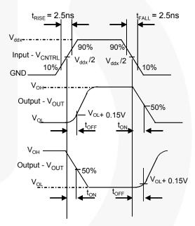
Figure 8. Turn On/Off Time Waveforms
