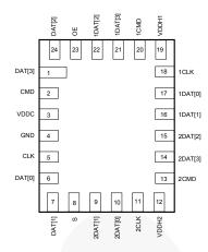
Figure 3. UMLP Pin Assignments
