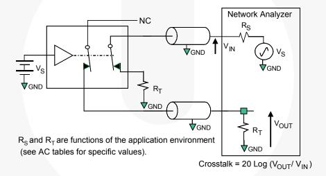
Figure 13. Channel-to-Channel Crosstalk
