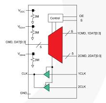
Figure 1. Analog Symbol Diagram
