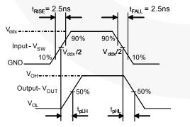
Figure 9. Switch Propagation Delay (tPD) Waveform
