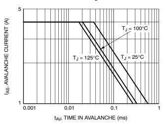
Figure 9. Unclamped Inductive Switching Capability
