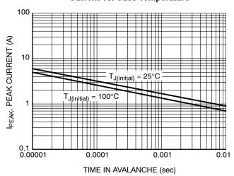
Figure 12. I<sub>PEAK</sub> vs. Time in Avalanche
