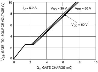
Figure 7. Gate-to-Source Voltage vs. Total Charge
