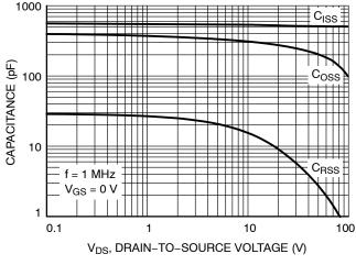
Figure 8. Capacitance vs. Drain-to-Source Voltage
