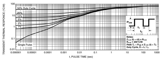
Figure 13. Transient Thermal Response Curve
