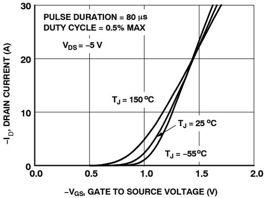
Figure 5. Transfer Characteristics
