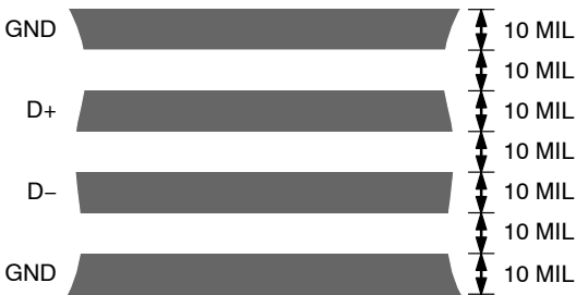
Figure 19. Arrangement of Signal Tracks
