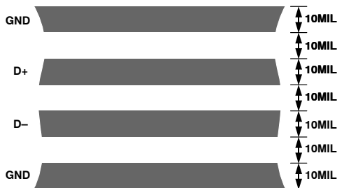
Figure 34. Arrangement of Signal Tracks
