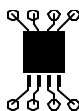
b) 125^\circ\text{W} when mounted on a 0.02\text{ in}^2 pad of 2 oz copper
