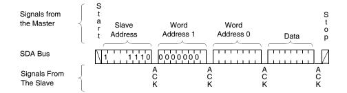
Figure 8. Writing 30 bytes to a 64-byte memory page starting at address 40.
