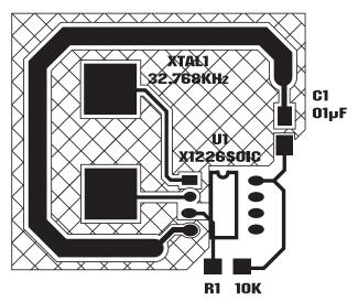
The X1 and X2 connections to the crystal are to be kept as short as possible. A thick ground trace around the crystal is advised to minimize noise intrusion, but ground near the X1 and X2 pins should be avoided as it will add to the load capacitance at those pins. Keep in mind these guidelines for other PCB layers in the vicinity of the RTC device. A small decoupling capacitor at the Vcc pin of the chip is mandatory, with a solid connection to ground.
