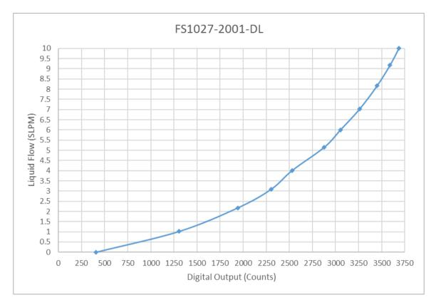
Figure 1. Digital Output Curve
